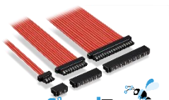
SignalBee™ DF52 Rated Current: 2.5A Max. Pitch: 0.8mm No. of Pos.: 2-20
