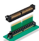
FunctionMAX™ FX27 Card Edge Connector Pitch: 0.8mm Stacking Height: 22mm Min. No. of Pos.: 40-120
