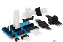
SignalBee™ DF51 Positive Lock (Side Lock) Rated Current: 3A Max. Pitch: 2.0mm No. of Pos.: 2-30
