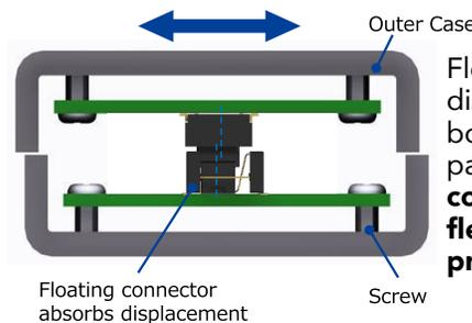
Floating design absorbs displacement between boards and stress to the panel from screws, **contributing to design flexibility in the end product.**
